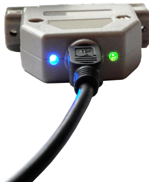
The 2 LEDs on the backshell of the UC100 controller.
