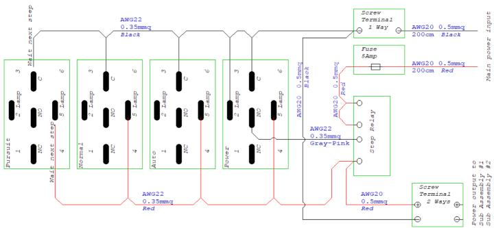
In this step we distribute both global power (that requires bigger gauge, thicker wires) and local power (that requires smaller gauge, thinner wires)
