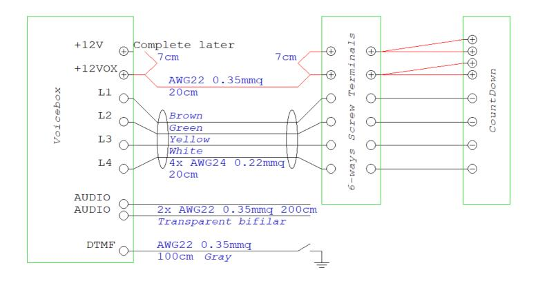
In this step we also perform local +12V power distribution. Use AWG22 = 0.35mmq red wire. Start daisy-chaining from the countdown screw terminals. A short 7cm between the position#5 and position#6 on screw terminals. Then continue with 20cm to +12VOX. Then continue with a short 7cm between +12VOX and +12V. Don't insert in +12V end, yet, but leave it floating. We will insert this in Step 3, because we have to continue the daisy-chain further, later.
